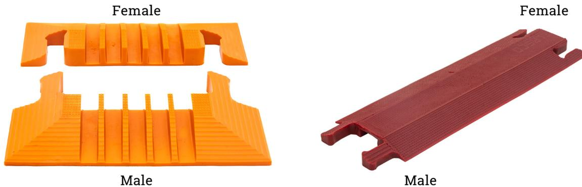
When placing the connection pieces together, always place the female side of top of the male side of the product (see above). Push down on the pieces at the connecting point using your hands or feet. When disconnecting the products, lift the female side upward. This applies to linear pieces, turns and end cap pieces.
